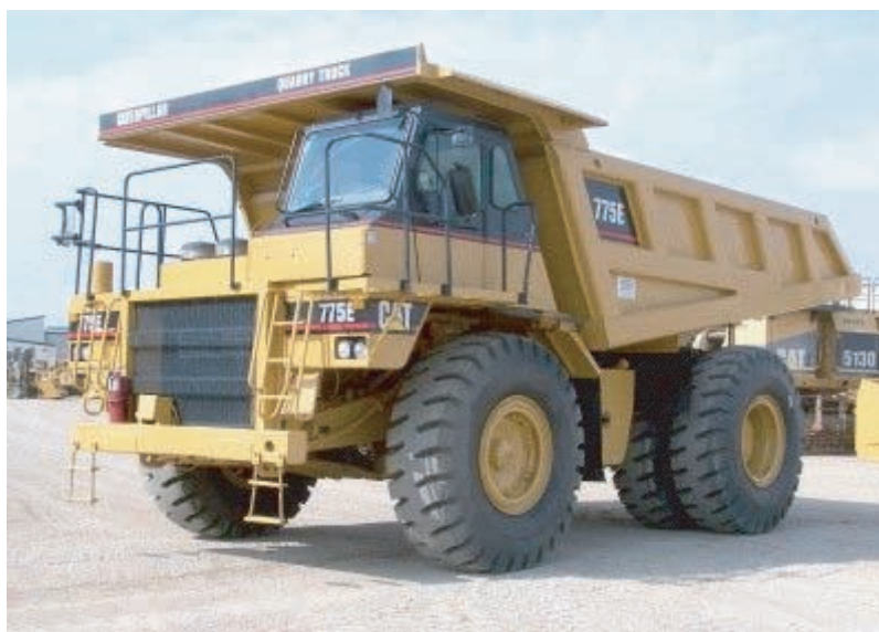
Figure 17.4. 64-tonne Caterpillar 775E Off-highway Truck
