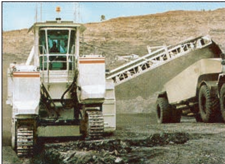
Figure 17.5. Wirtgen surface miner
