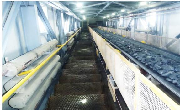
At Mill-4, the installation of an additional conveyor to transport pebble to the large cone crusher bypassing the first stage pebble crusher. This initiative allowed to avoid a decrease in productivity during the first stage cone crusher downtimes and to stabilize the ore feed preparation process
